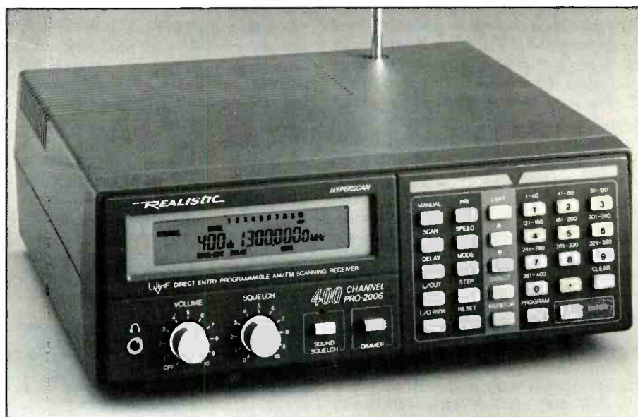
Several of today's more sophisticated scanners (like this Realistic PRO-2006) can tune in the exciting 225 to 400 MHz military UHF aero band.
